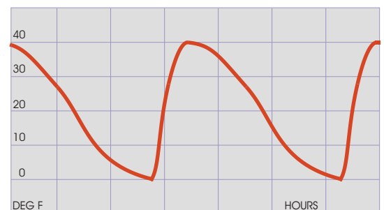
Freeze-thaw cycle profile can be customized to meet specific test parameters, as shown above.
